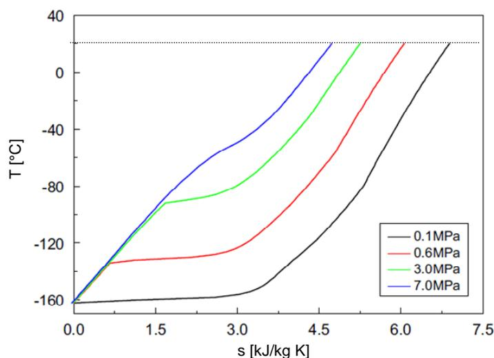
**Figure 1.** T-s diagram for LNG
