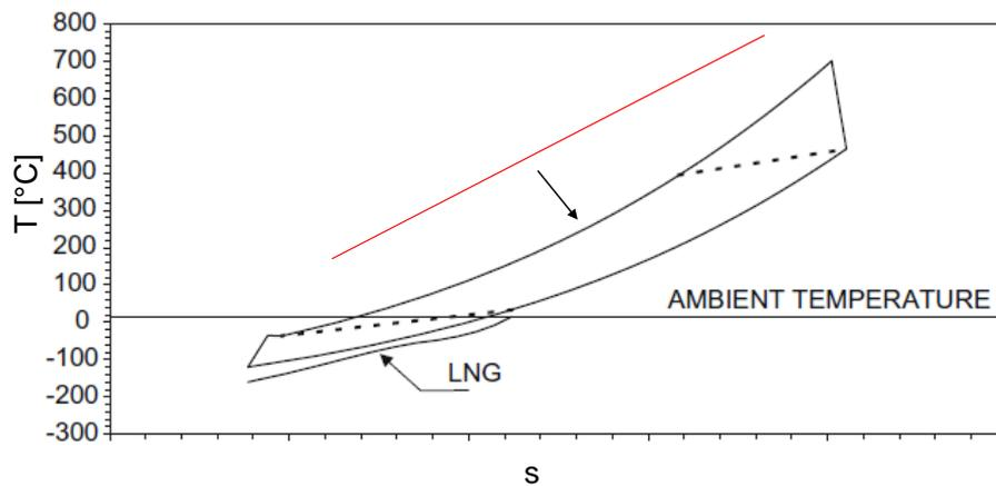
**Figure 5.** The cooling capacity of supercritical LNG in relation to high temperature Brayton cycle
