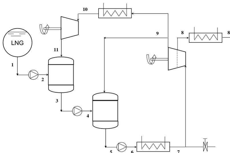
**Figure 6.** Direct expansion cycle configuration analyzed
