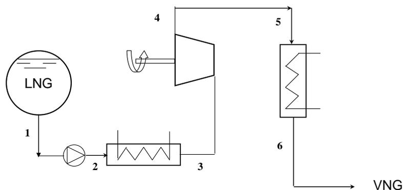
Figure 2. Direct expansion cycle
