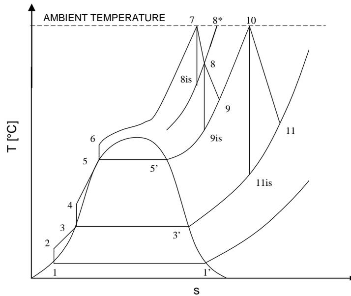
**Figure 7.** Direct expansion cycle considered: schematic T-s diagram
