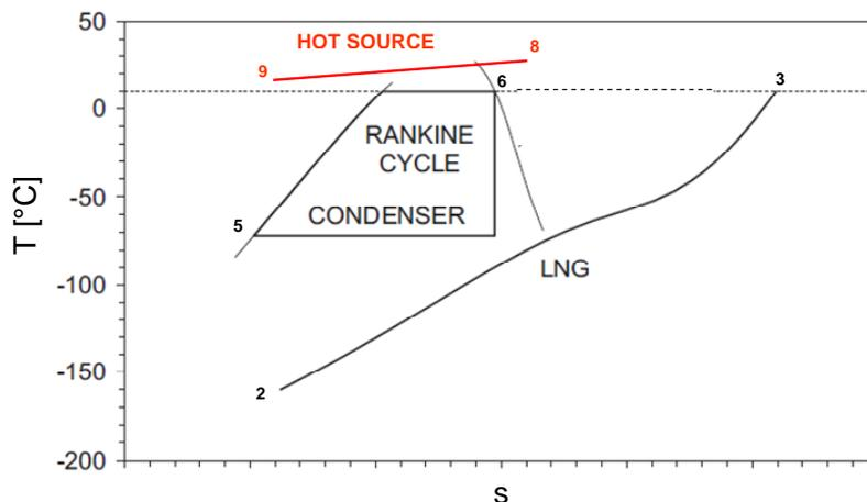
**Figure 4.** The cooling capacity of supercritical LNG in relation to Rankine cycle
